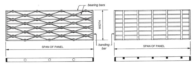
SPAN of panel is measured parallel to the bearing bars.
