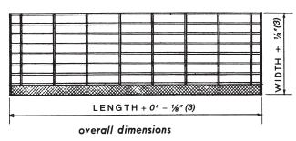
NOTE: Length of tread is distance between outer faces of carrier plates or back to back of carrier angles.
