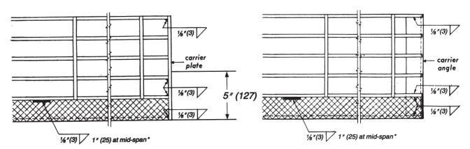
When carrier plates are used, the bearing bars and the nosing in the front five inches shall be welded to the carrier plate as shown.
