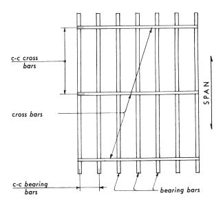
WELDED OR PRESSURE-LOCKED GRATING
