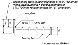
load-carrying toe plates toe plate
